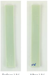
ISO 4892-1/4892-2: Xenon-arc lamp, UV-Quartz filter, 1.2  $\mbox{W/m}^2\mbox{/nm}$ , at 420 nm, 70 °C, 6 hours
