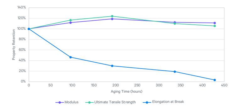
ASTM 4459: Q-Sun XE-1, 0.8 W/m²/nm at 420 nm, 55 °C ASTM D638: Type V, 10 mm/min, average values represented
